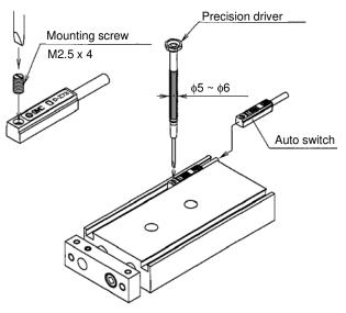
M2.5 mounting screw tightening torque must be 0.05 to 0.1 Nm
