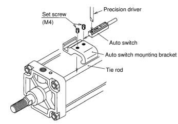
M4 set screw tightening torque must be 1.0 to 1.2 N•m.
