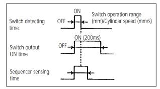
• To use the auto switch as an intermediate stop signal, the position of the switch must be adjusted to take into account the speed of the actuator, i.e. over travel of the stopping position during braking applications.
