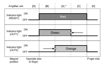
\* Dimension for [A] should be 0.5 mm minimum in the stroke direction.
