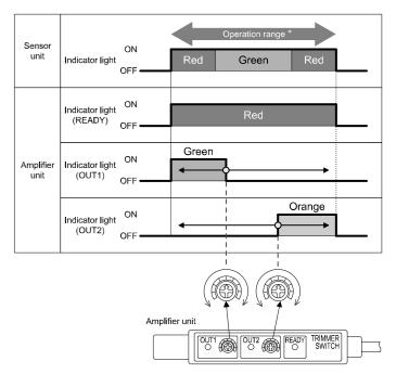
\* For standard products, the operating range depends on the actuator and bore size. It cannot be varied
