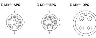
M8-3 pin connector M8-4 pin
