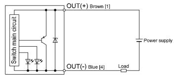
The number shown in brackets [] in the wiring diagram indicates the prewired connector pin number.
