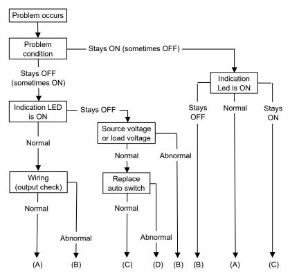
(A) = Auto switch output failure (replace)
