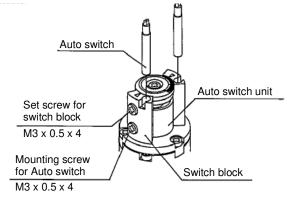
• Loosen the switch mounting screw in the auto switch unit and insert the auto switch. Tighten the mounting screw.
