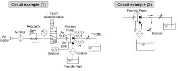
Fig 2. Automatically Operated Circuit Examples
