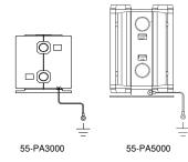
Fig.1 Method of Connecting Ground Cable
