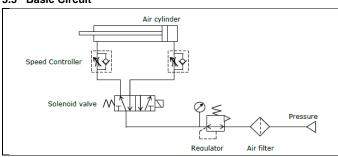
Plugging one of the ports on the actuator is considered a non-intended use, and could relate to an increase in maximum surface temperature above what the product specification declares.
