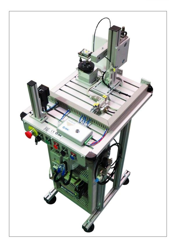
The system inspects bearing height, shaft material, lid height and material and the tightening torque of the four screws forming the assembly.
