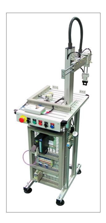
The station is formed by a 450x600x900mm height-adjustable aluminium structure, on which the components used to perform the process are mounted, which include a block of control solenoid valves in the case of pneumatic components.
