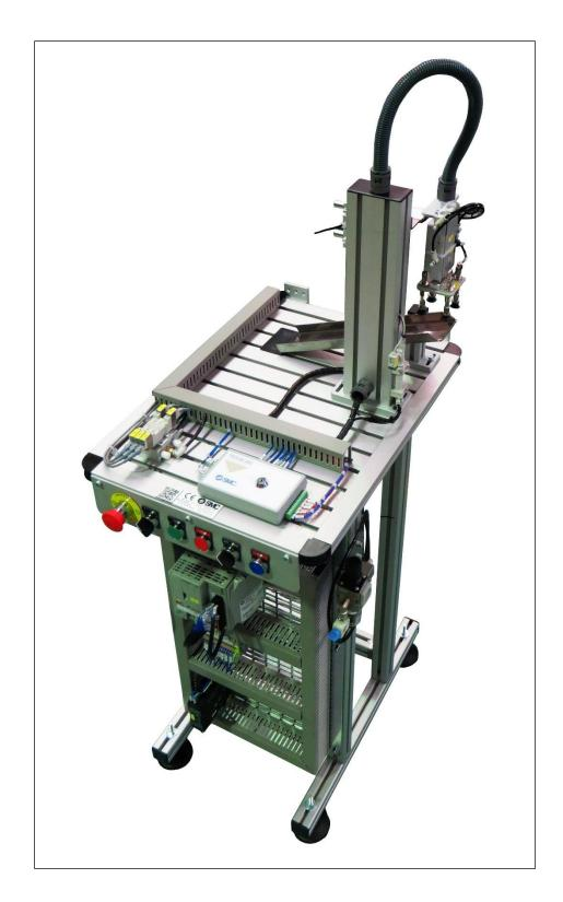
The station is formed by a 450x600x900mm height-adjustable aluminium structure, on which the components used to perform the process are mounted, which include a block of control solenoid valves in the case of pneumatic components.
