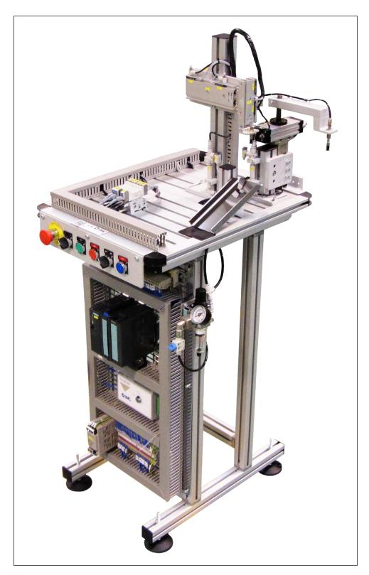
The part to be assembled is a shaft, 14.6mm diameter and 41mm height. There are two shaft insertion options: metal shaft, anodised aluminium shaft and plastic shaft, made from black nylon.
