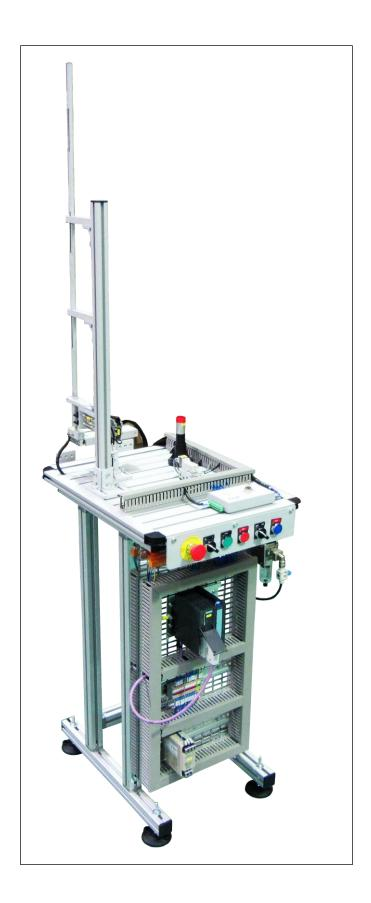
The station is formed by a 450x600x900mm height-adjustable aluminium structure on which the components used to perform the process are mounted,
