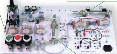
Components with connectors for 4mm tube
